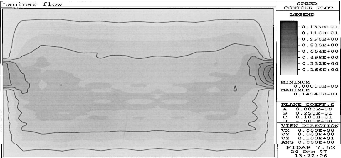
Fig. 3 Speed contour for the middle slice (0.9 m), laminar flow.
